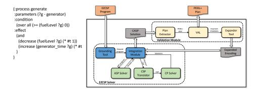
Fig. 1. PDDL+ process from the generator domain (*left*); Extended solver architecture (*right*).
