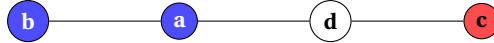
Fig. 1: The undirected graph used as running example. Source vertices in blue, sink vertex in red. The goal is to assign directions to edges so that all source nodes still reach all sink nodes.
